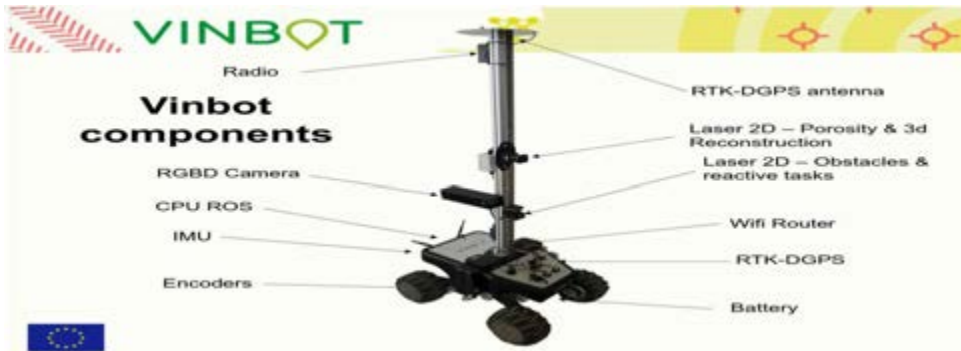
Figure 2. VinBot- distribution of components
